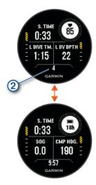
**Surface interval screen**: Displays the current surface interval time, as well as the elapsed time, maximum depth, and temperature for your last apnea dive. You can edit the data fields.
