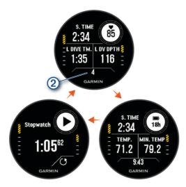
**Surface interval screen**: Displays the current surface interval time, heart rate, and last dive information. You can edit the data fields.
