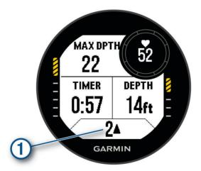
**In-dive screen**: Displays the information about the current dive, including the elapsed time, current and maximum depth, heart rate data, and rate ascent or descent. You can edit three of the data fields (*Customizing the Data Screens*, page 40).
