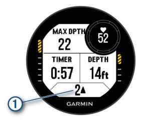
**In-dive screen**: Displays the information about the current dive, including the elapsed time, current and maximum depth, heart rate data, and rate of ascent or descent. You can edit three of the data fields (*Customizing the Data Screens*, page 40).
